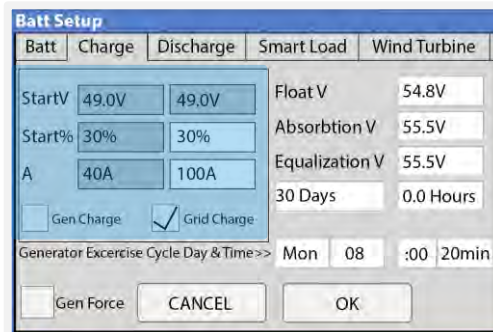
Generator and grid charge settings
