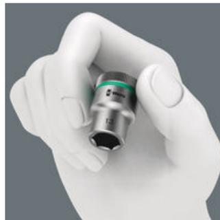
The Zyklo sockets are suitable for manual and machine-operated tools (non impact). They feature a ball stop groove and knurling at the rear end for manageability during manual use. They are made of chrome-vanadium, matte-chromed. Take it easy tool finder: colour coding by size as well as size stamping - to help you find the required socket quickly and easily.
