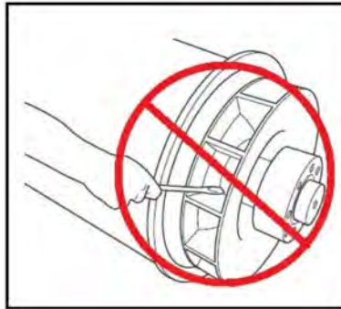
FIGURE 39. DO NOT ROTATE ROTOR USING FAN
